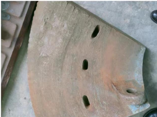
Ceramic insert casting spirall liner After 4 months of use Ceramic insert casting spirall liner after 4 months of use
