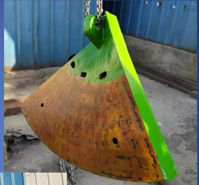
陶瓷复合立式螺旋搅拌磨机(塔磨机)螺旋衬板 ceramic insert spiral liner of Vertical spiral agitating mill (towermill, SMD)
