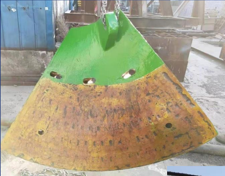
陶瓷复合立式螺旋搅拌磨机(塔磨机)螺旋衬板 ceramic insert spiral liner of Vertical spiral agitating mill (towermill, SMD)
