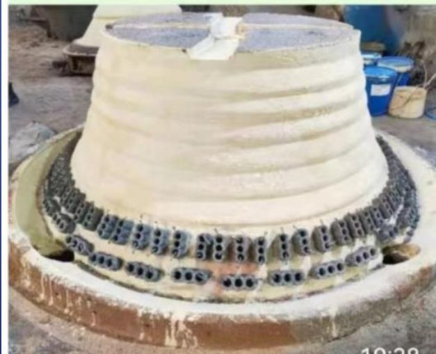
high manganese steel ceramic insert casting Cone
