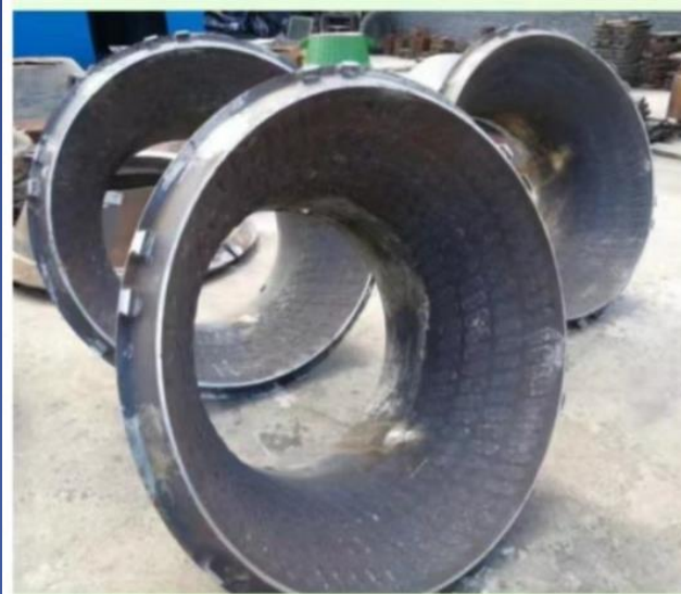
high manganese steel ceramic insert casting Cone
