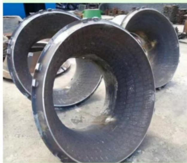
high manganese steel ceramic insert casting Cone
