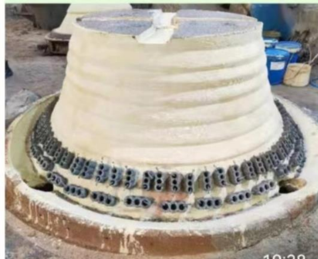
high manganese steel ceramic insert casting Cone
