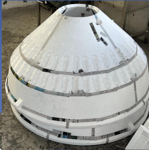
消失模铸造工艺高锰钢陶瓷复合轧白壁陶瓷布局及安装 installation and layout of Ceramic core for high manganese steel ceramic insert casting Mantle / Bowl of Lost foam casting process
