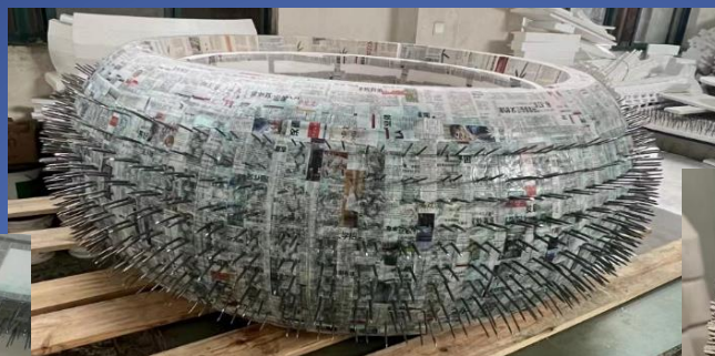
消失模铸造工艺高铬陶瓷复合辊套的陶瓷布局及安装 installation and layout of Ceramic core for high Chrome cast iron ceramic insert casting Roller of Lost foam casting process
